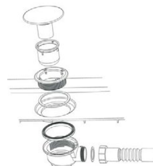
Installation of siphon
