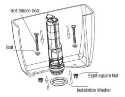
3. Take the Body of Flush valve back to Base and rotate it clockwise. Knot Installation washer to Round nut and put Tank on the right place of Bowl. Then insert Tank to Bowl bolt with Bolt silicon seal in the bolt hole (as picture) and screw Eight-square Nut to Tank to Bowl Bolt tightly.
