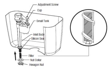
Unscrew Hexagon nut and Nut collar from the Fill valve, insert Fill valve with Silicon seal into the inlet hole of Water tank and make sure Fill valve is in the right position, then screw Nut collar and Hexagon nut in turn to Fill valve tightly. Then connect Refilling tube with the Overflow pipe of Flush valve.
