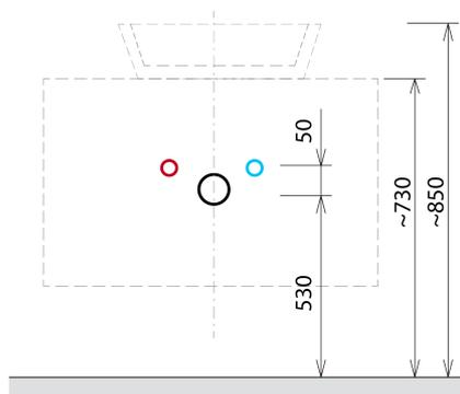
Installation of drain + hot & cold water pipes
