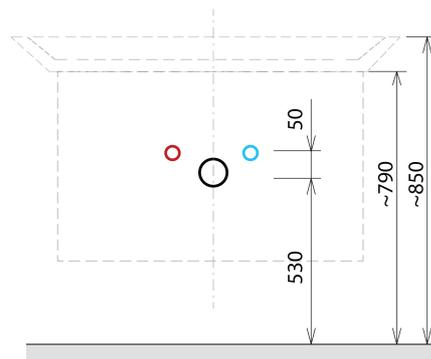
Installation of drain + hot & cold water pipes
