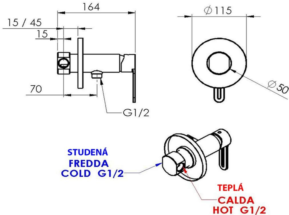
**PRŮTOK / PORTATA / FLOW RATE = 8 l/min**
